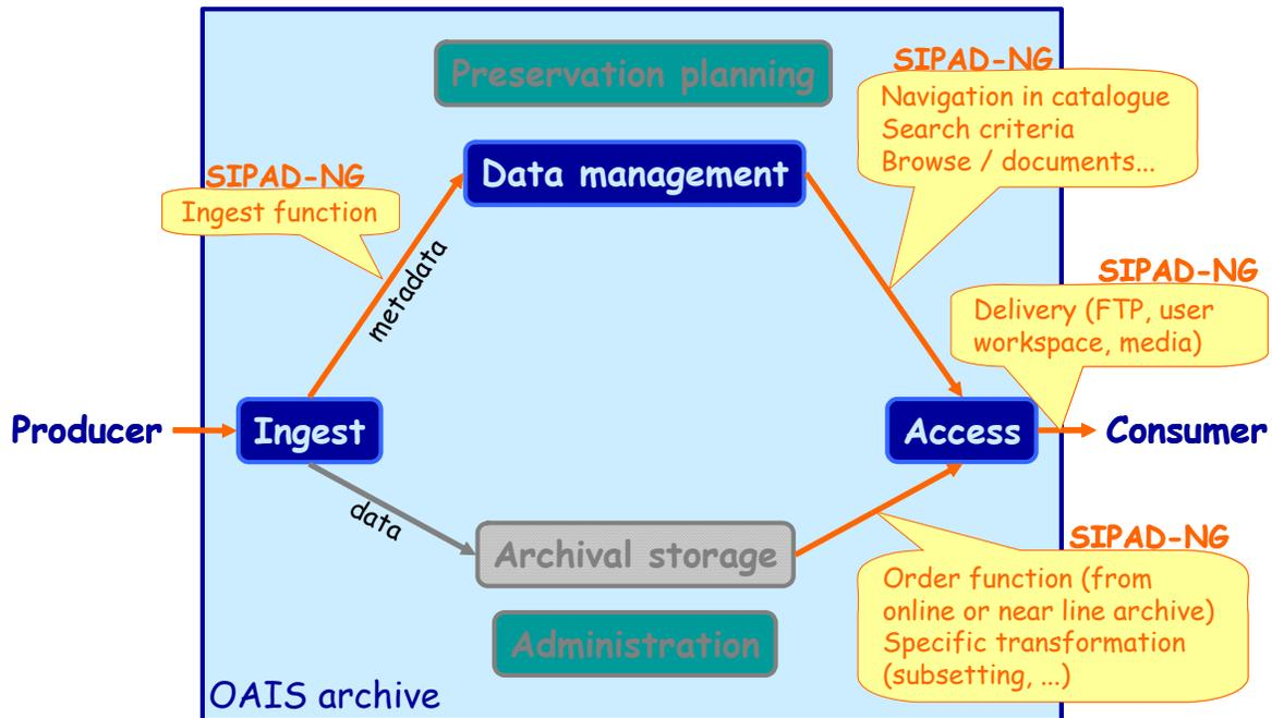
Figure 5: OAIS functions implemented by Sipad-NG to meet Data Centres requirements
