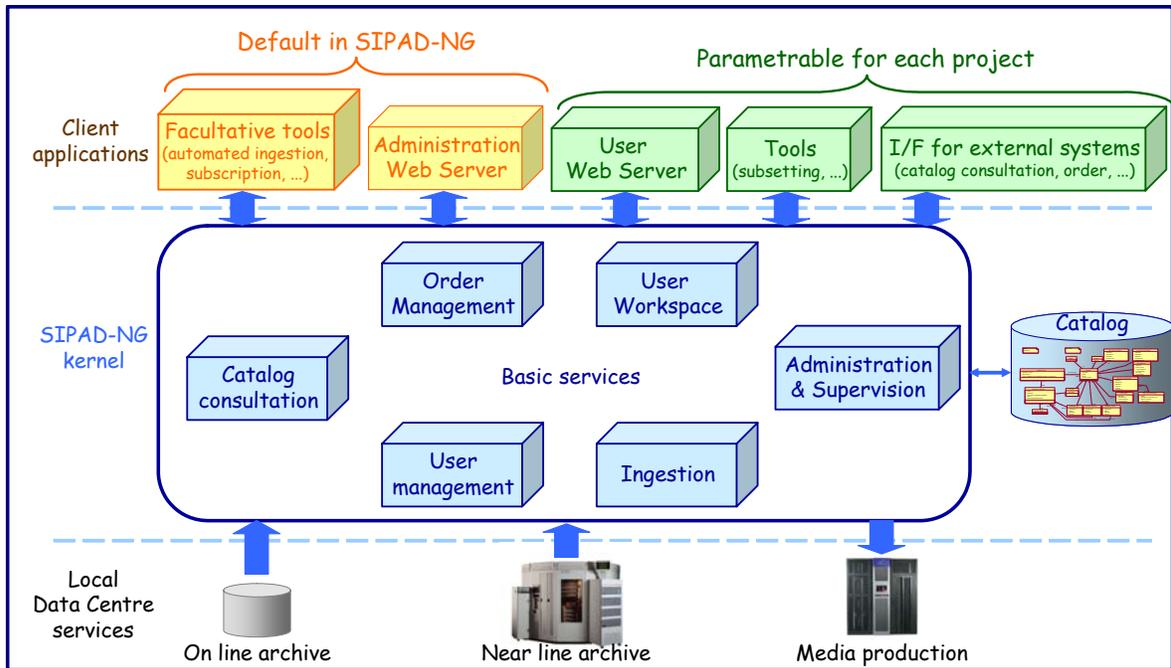
Figure 6: Sipad-NG architecture – client applications interface “basic services” that share information through a relational database
