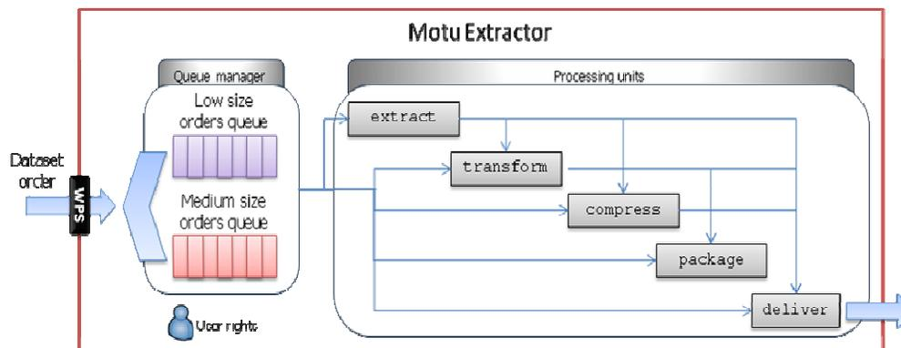
Figure 10: Internal logical view of Motu Extractor
